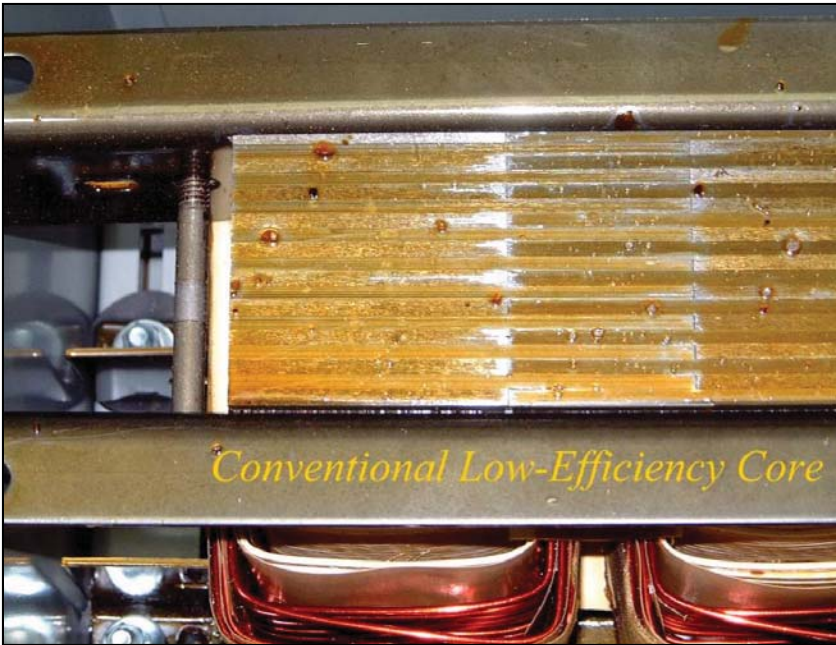
Figure #7—Picture of the core construction of a standard transformer. This core construction incorporates thicker laminations.
